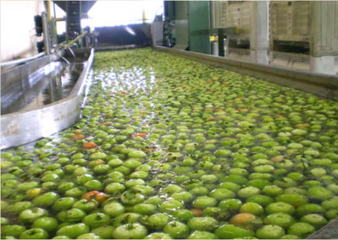
Dump Tank Bin Wash
