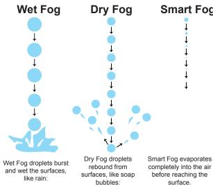
**Smart Fog** "Smart Fog is a fog that does not moisten the exposed surfaces"
